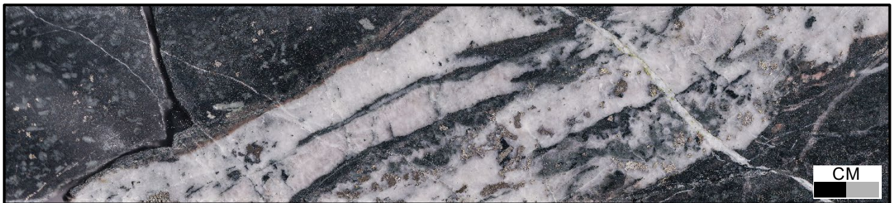
Figure 6: SPD029 58m grading 3.75 g/t Au . Laminated carbonate-pyrite-chalcopyrite-chlorite vein overprinted by carbonate-epidote vein in monzonite with disseminated pyrite halo.
