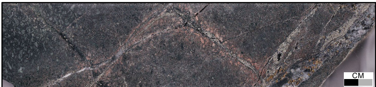
Figure 7: SPD030 165m grading 13.68 g/t Au . Multiple generations of sulphide veining. Vuggy quartz-bornite-magnetite-chalcopyrite vein reactivating a pyrite sulphide vein and crosscutting earlier pyrite veinlet with potassic selvage. Late carbonate-chlorite-pyrite vein in monzonite.
