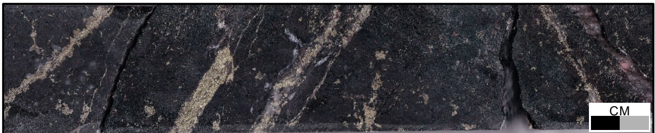
Figure 2: SPD025 491m grading 47.81 g/t Au . Pyrite, Chalcopyrite and pyrite-chalcopyrite veinlets, quartz-pyrite-chalcopyrite veins and disseminated pyrite in basalt.
