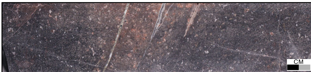
Figure 4: SPD024 512.2m grading 1.59 g/t Au. Pyrite-carbonate and quartz-pyrite veins in weakly potassic altered andesite.
