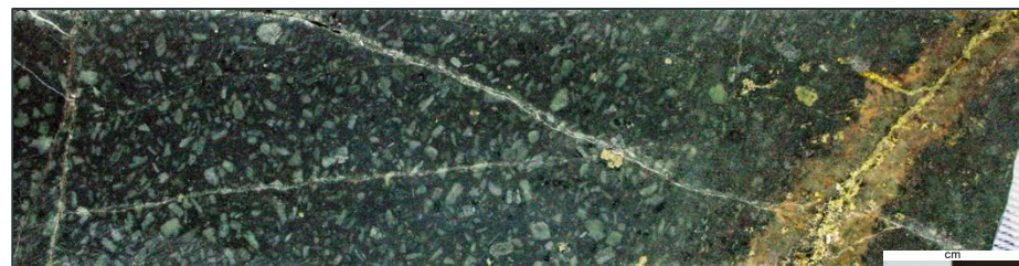
SPRCD062 669.7m – Veinlet chalcopyrite + quartz ± pyrite with strong k-feldspar vein halo, 43.3g/t Au
