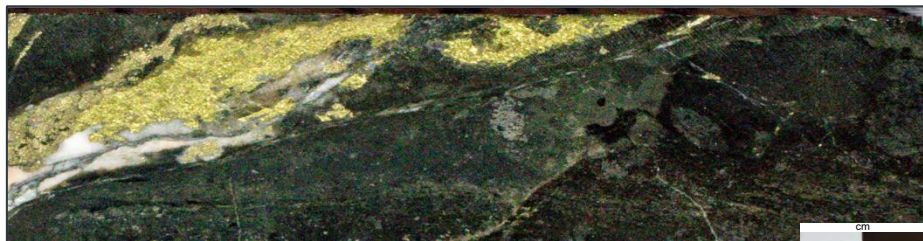
SPRCD062 616.9m – Stringer chalcopyrite + quartz ± pyrite with pervasive chlorite alteration, 8.39g/t Au
