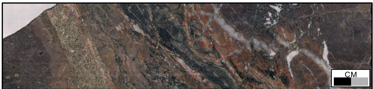
Figure 7: SPD086 at 72.2m, 1m @ 0.69 g/t Au.
