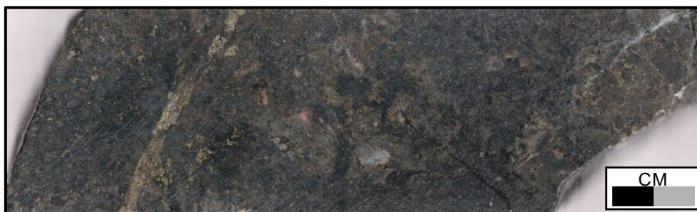
Figure 6: IDD001 at 650.2m, 1m @ 3.95 g/t Au.
