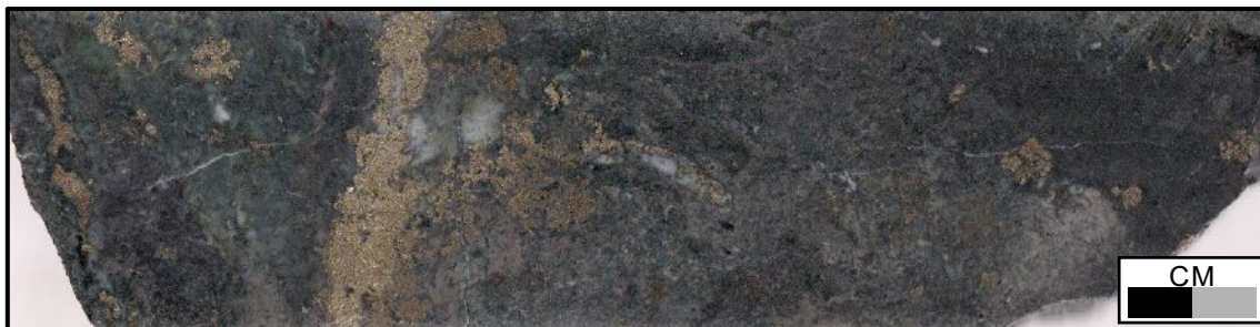
Figure 5: IDD001 at 636.2m, 1m @ 5.83 g/t Au.
