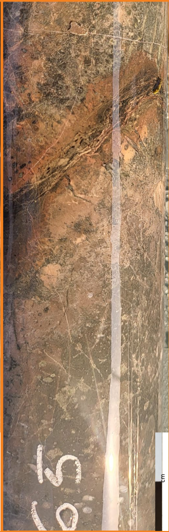
SPD001 - 265m, strong, vein-controlled, k-feldspar alteration (Inner Propylitic Porphyry Alteration)
