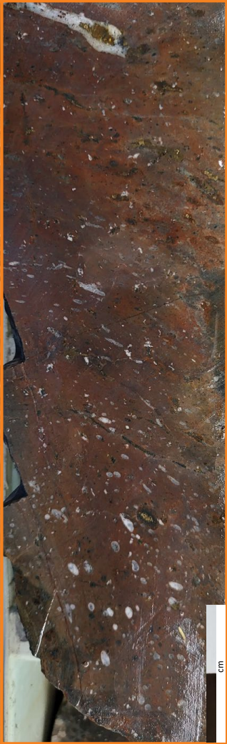
SD010 - 160m, massive hematite + silica (red-rock) alteration, pyrite-chalcopryrite stringers, 0.82g/t Au (Inner Prop Porphyry)
