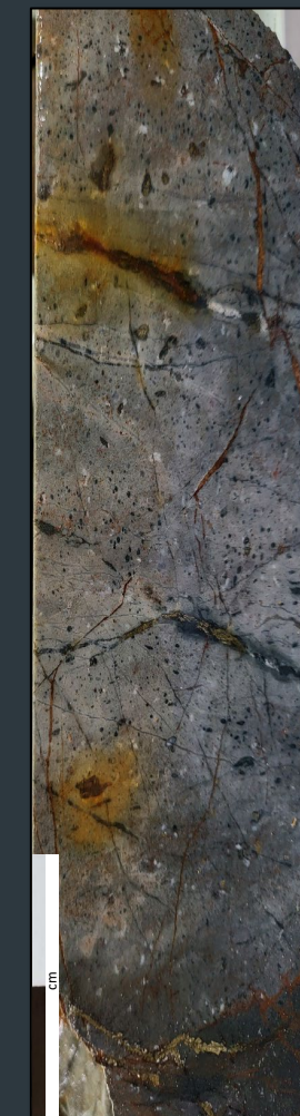
K-spar + albite + silica + tourmaline alteration, 2g/t Au, 0.14% Cu (Alkalic lithocap porphyry alteration, SD010 – 196m)
