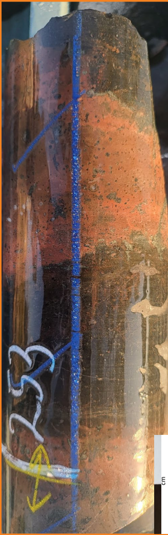
SPD001 - 253m, strong k-feldspar alteration (Inner Propylitic Porphyry Alteration)
