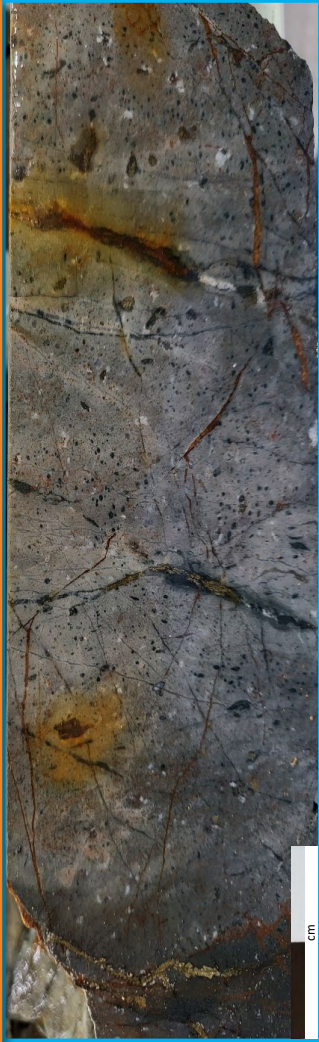
SD010 - 196m, massive kspars + albite + silica + tourmaline alteration + pyrite-chalcopryrite stringers, 2g/t Au, 0.14% Cu (Alkalic lithocap Porphyry)
