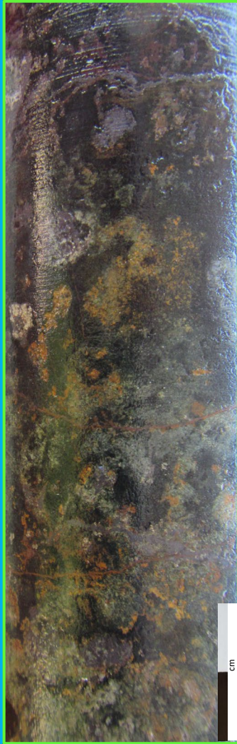
SPD001 - 24.2m, hematite + epidote-pyrite skarn, 22m @ 1.92g/t Au from 11m, inc 5m @ 6.69g/t Au (Oxidised Retrograde Skarn)
